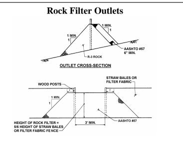
Sediment must be removed when accumulations reach 1/3 the height of the outlet.
