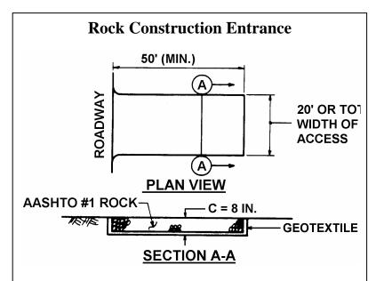
MAINTENANCE: Rock Construction Entrance thickness shall be constantly maintained to the specified dimensions by adding rock. A stockpile shall be maintained on site for this purpose. At the end of each construction day, all sediment deposited on paved roadways shall be removed and returned to the construction site.
